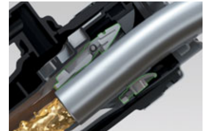
When the larger diesel fuel nozzle is inserted, the interlock opens to allow fueling.
