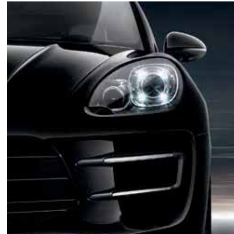
Daytime running lights with Bi-Xenon™ headlights
